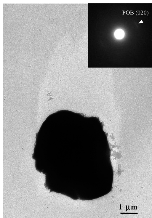
Figure 9. Shadowed image of a spindlelike crystal prepared from ABA and APBA at \chi_f of 10 mol % for 1 h.
